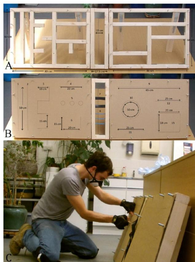
Figure 4. The wooden frame securing the materials in place (A), the lengths of cardboard, rope and neoprene cut (B), and an initial trial run of the experiment (C).
